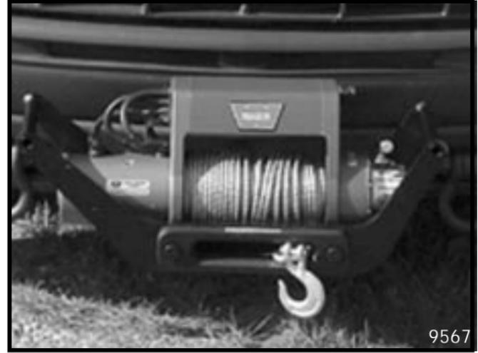
The multi-mount winch has 9,000 lbs (4082 kg) of single line pull. The multi-mount slides into the hitch receiver and allows you to move and operate the winch from the front or the back of vehicle.
