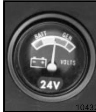
The voltmeter needle should be between the yellow and the green bands in a no load situation.
