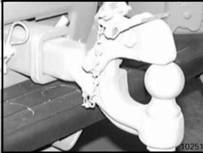
A pintle hitch is located at the rear of the vehicle, and is removable from the receiver.
