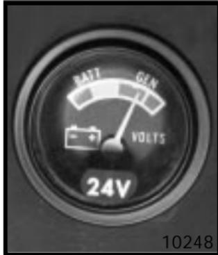
The voltmeter needle should be in the green band during normal load operation. If the needle is not in the green band, the fuse may have blown. If the fuse is not blown and the system still does not work properly, report it to your maintenance support activity.
