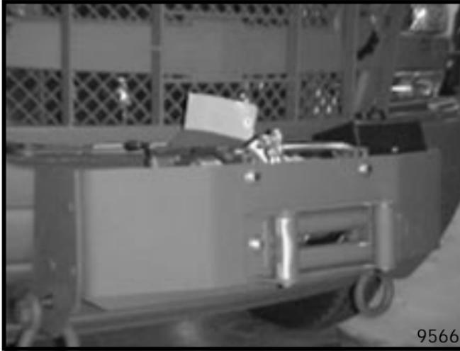
The winch is electrically powered from the vehicle batteries. The permanent mount winch has 12,000 lbs (5440 kg) of single line pull.
