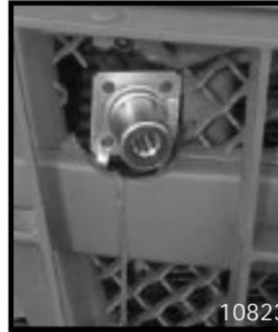
3. Locate the slave receptacles on both vehicles and unscrew the cover.
