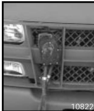
4. Connect the slave cable to the vehicle with the dead battery.
