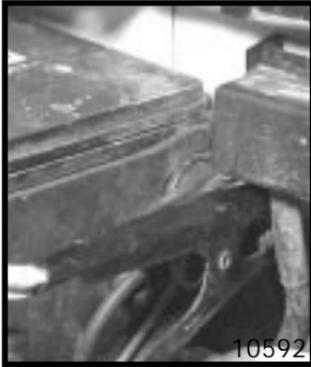
6. Connect the negative (-) cable to the negative (-) post of the 12-volt system of the vehicle with the good battery.
