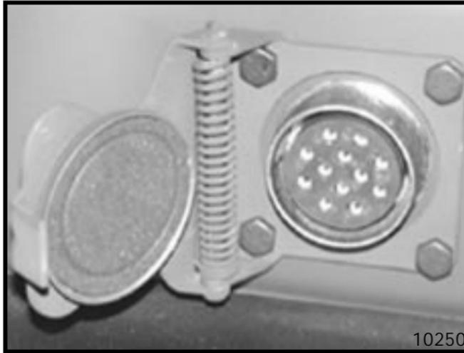
The NATO standard 12-pin trailer lamp and brake connector is located on the rear bumper to the right of the pintle hitch, or on the hitch receiver to the left of the pintle hitch.
