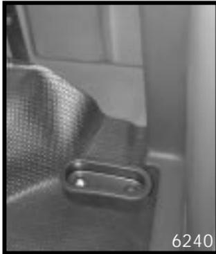
To secure weapons in the vehicle, first place the stock in the lower weapon support.
