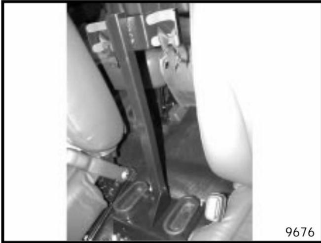
On Tahoe/Suburban models, place the barrel into the upper weapon support. Pull the strap outward and slide it over the barrel of the rifle and secure buckle.
