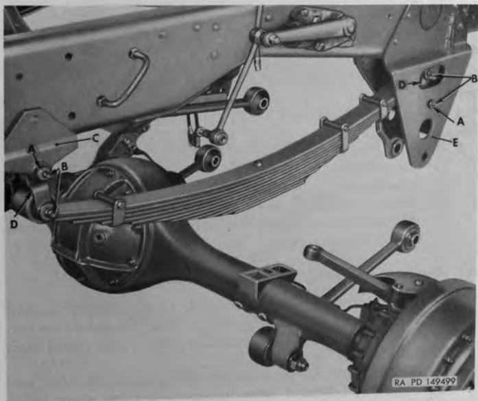
Figure 34. Front spring disconnect points.
