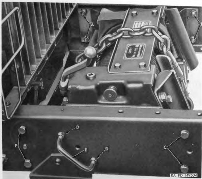
Figure 17. Winch disconnect points.
