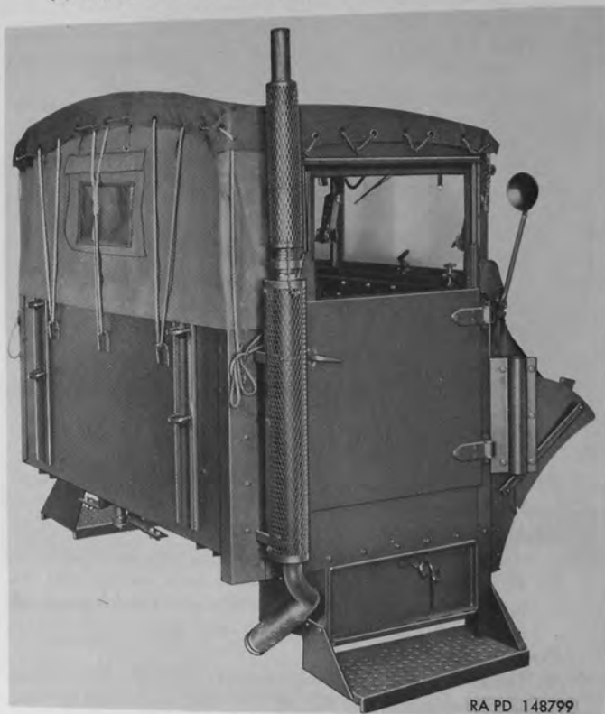
Figure 20. Cab assembly removed.
