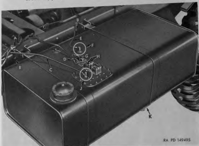
Figure 24. Fuel tank disconnect points.
