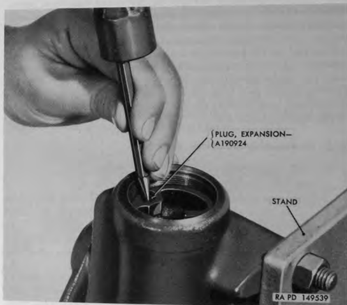
Figure 209. Removing piston screw expansion plug with shock absorber mounted in stand 41-S-4977-5.
