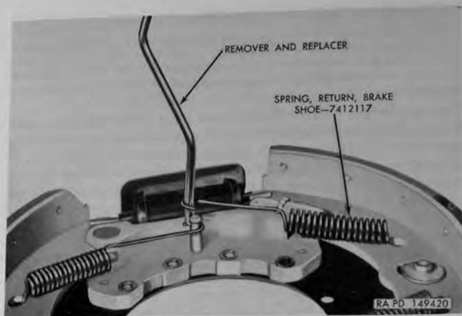
Figure 167. Installing brake shoe return springs with remover and replacer 41-R-2375-20.
