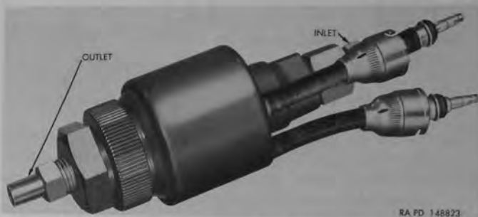
Figure 177. Overall view of temporary (electric) parking brake valve.
