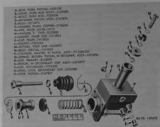
Figure 168. Master cylinder components.
