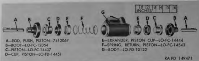
Figure 171. Wheel cylinder components.
