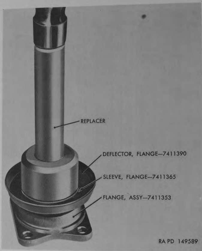
Figure 156. Installing flange oil seal sleeve with replacer 41-R-2395-528.
