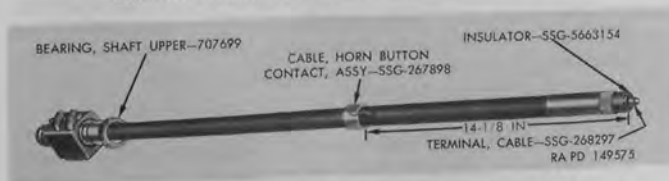
Figure 197. Construction of steering shaft assembly.
