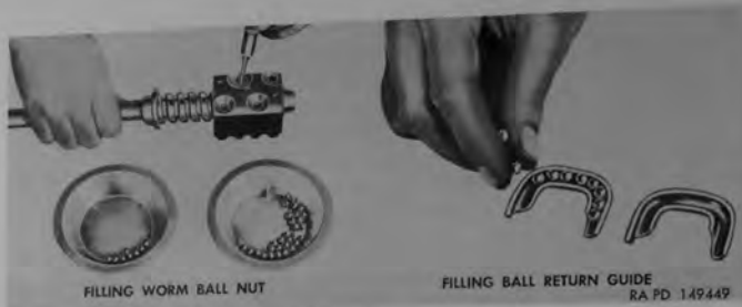
Figure 199. Installing worm balls into worm ball nut and return guides.
