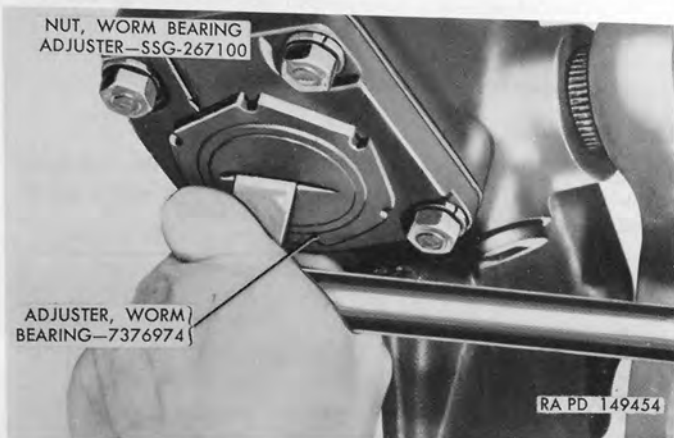
Figure 202. Adjusting worm bearings.
