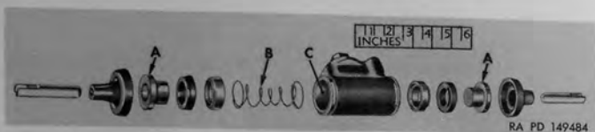
Figure 251. Repair and rebuild standard points of measurement for wheel cylinders.
