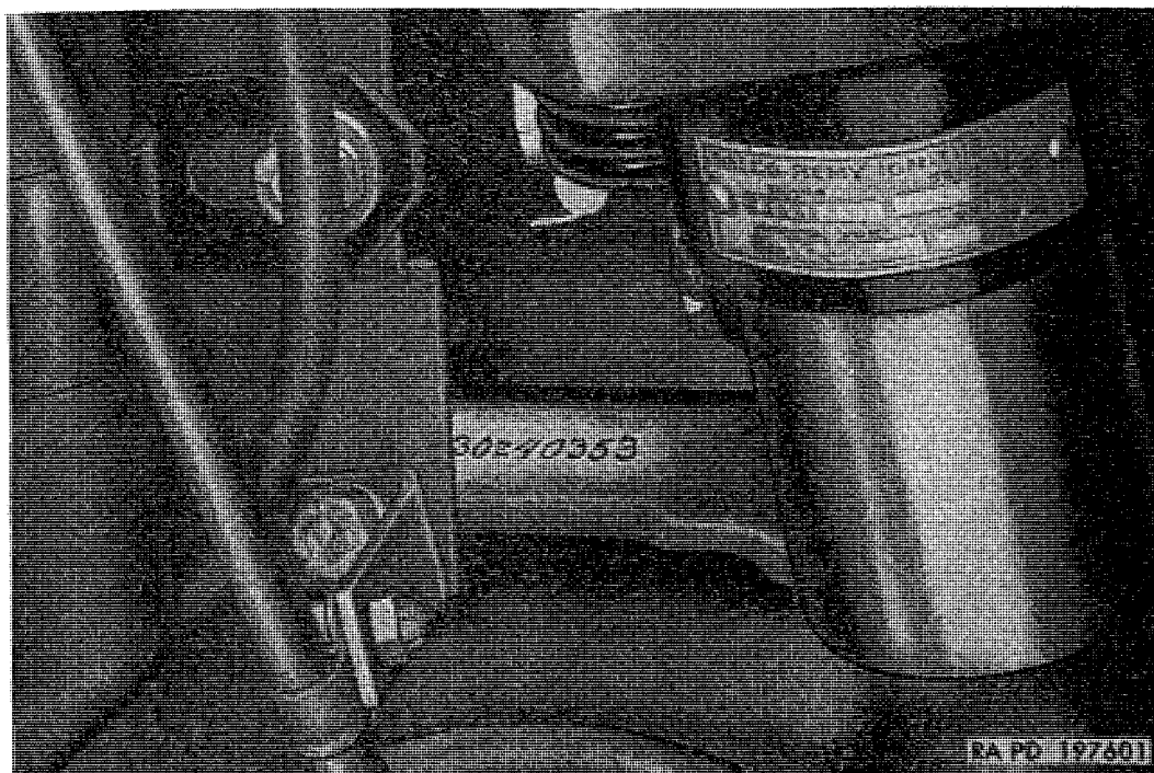
Figure 25. Engine serial number stamp location.
