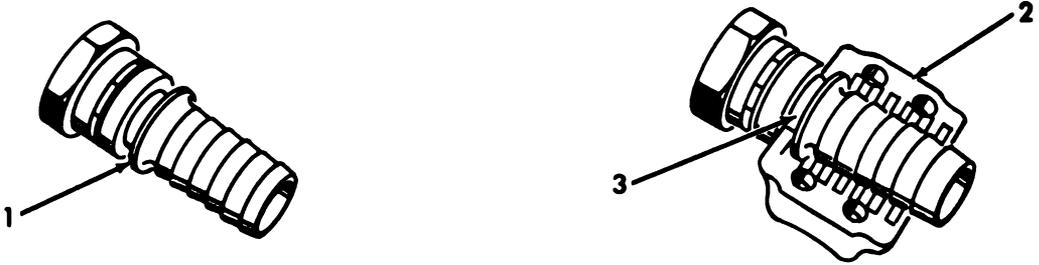
Place Clamp halves (2) over hose with clamp front collar in nipple channel (3).
