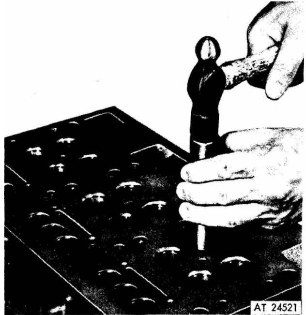
Figure 8. Installing exhaust valve seat insert.
