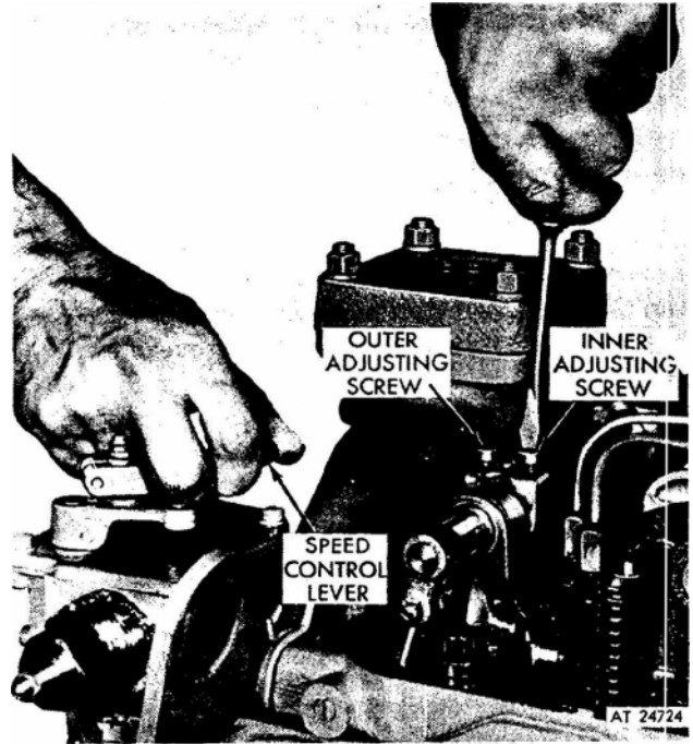
Figure 2. Positioning the rear injector rack control
