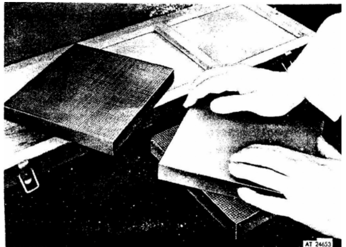
Figure 1. Refinishing lapping blocks.
