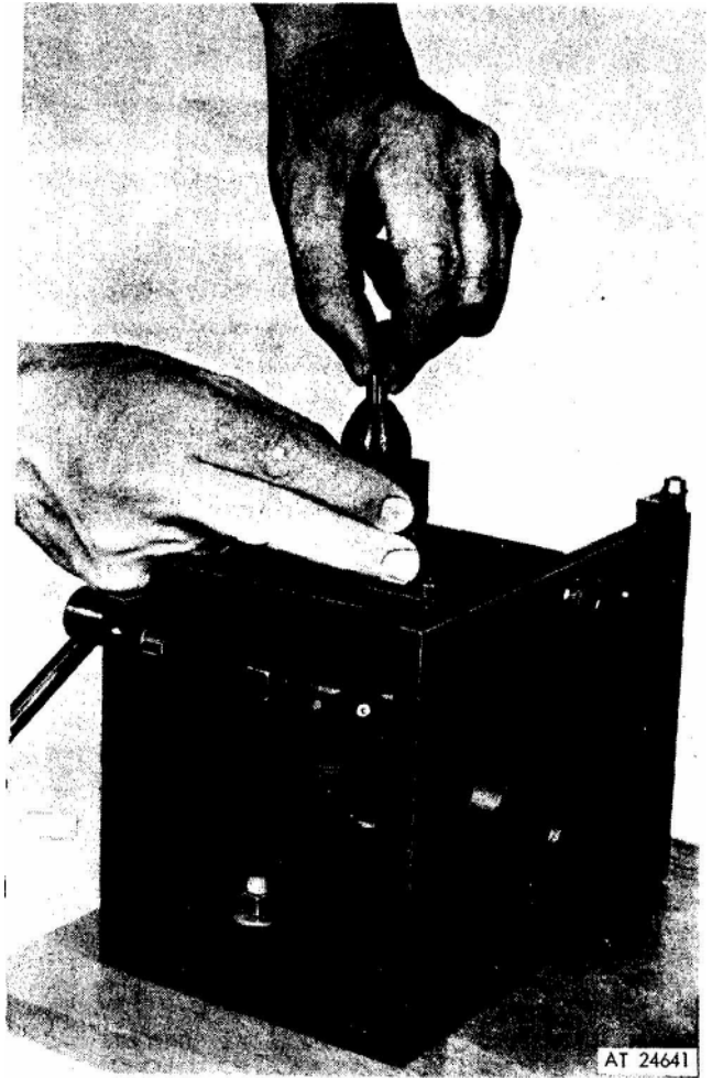
Figure 33. Tightening injector nut by hand
