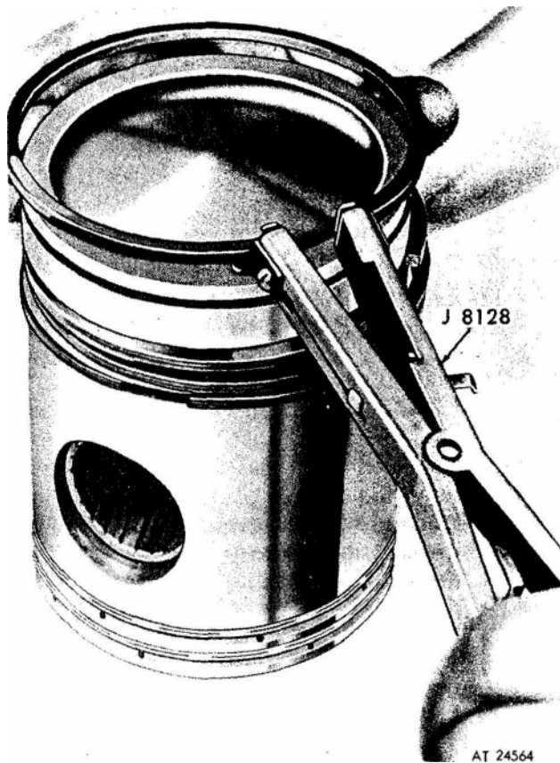
Figure 2. Removing or replacing piston rings.
