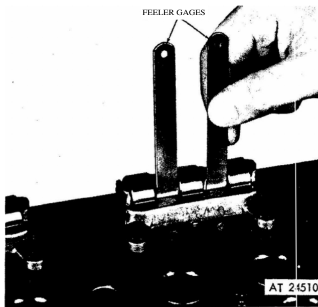
Figure 9. Checking the clearance between the cam follower guide and cam follower legs.
