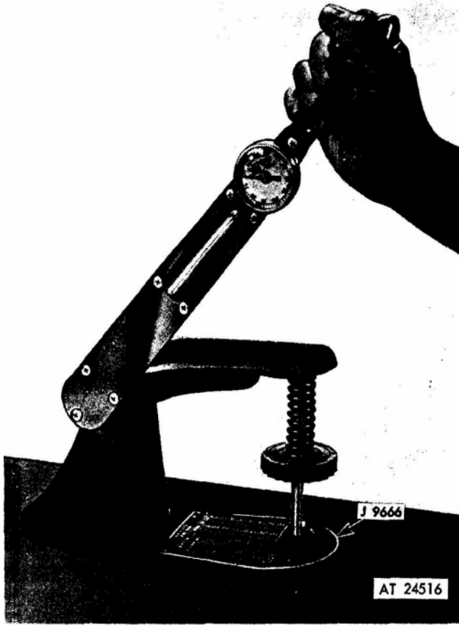
Figure 3. Testing exhaust valve spring
