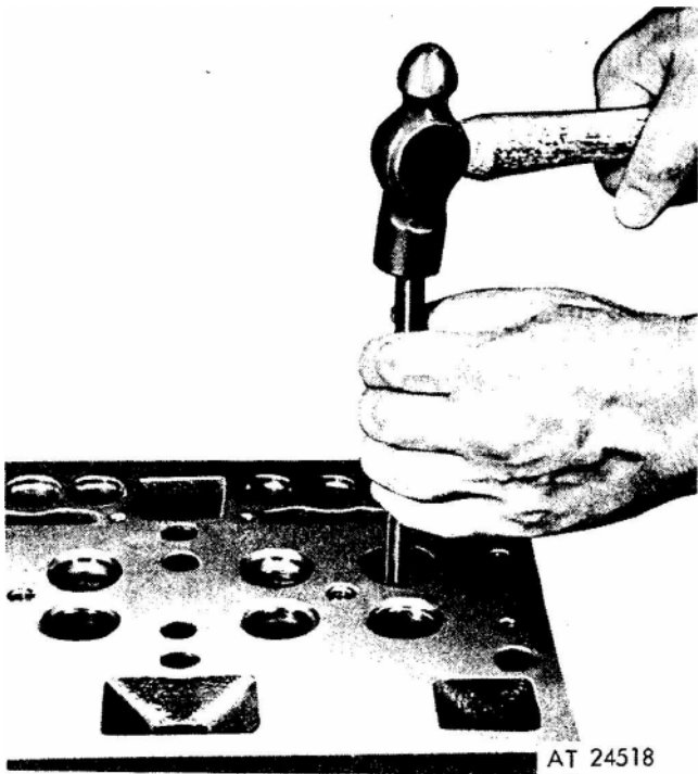
Figure 5. Removing exhaust valve guide.
