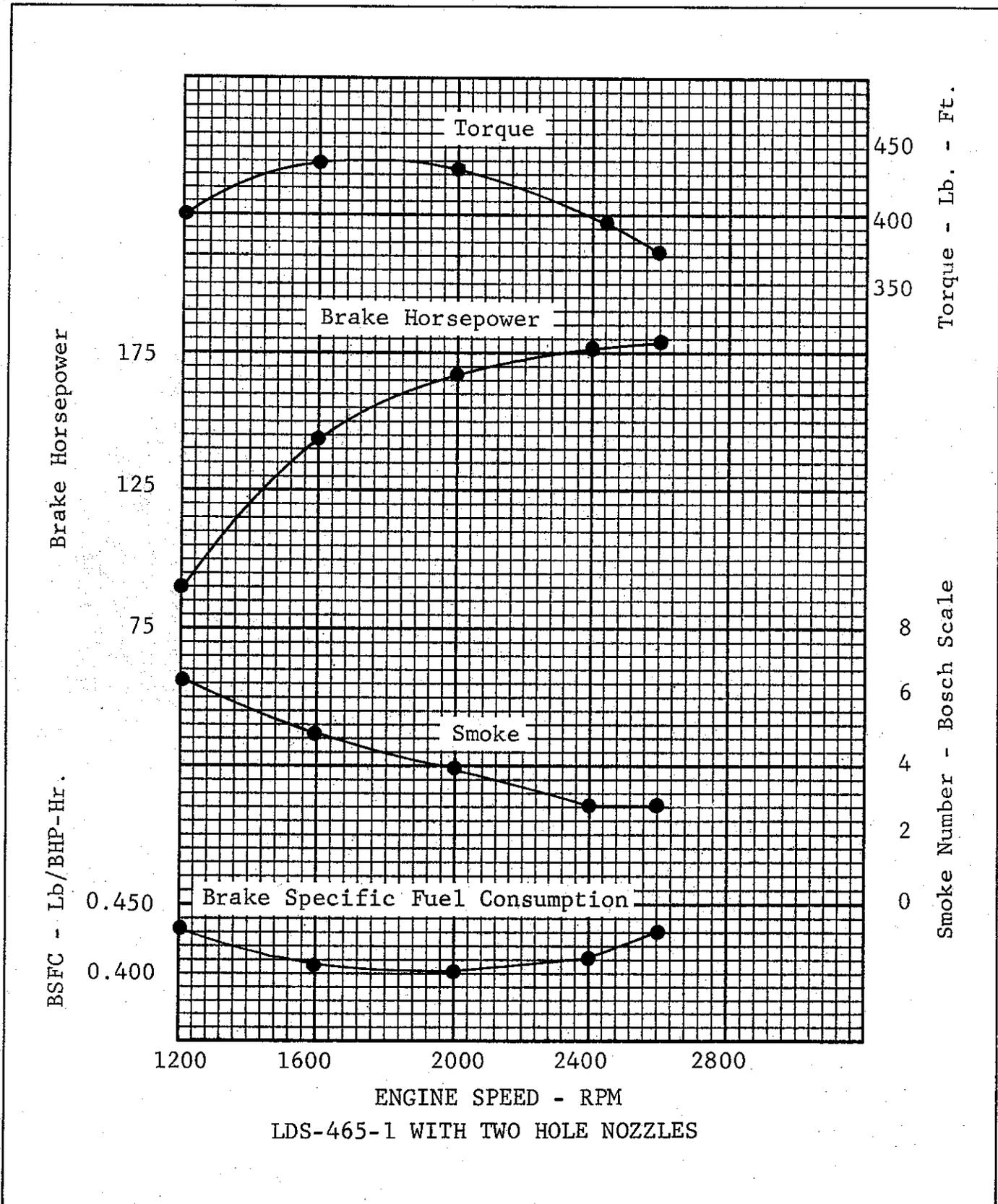
Figure 1. Performance Curve, LDS-465-1 Engine With Two Hole Nozzles
