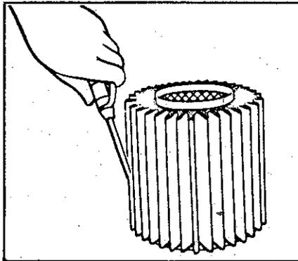
F. Blow off the outside of the cartridge with 100 lbs. compressed air.
