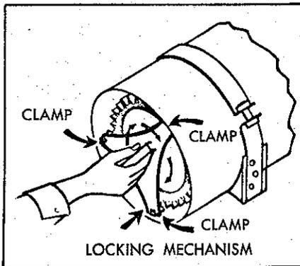
J. Replace locking mechanism by turning mechanism to engage under clamps. Tighten by turning handle clockwise.
