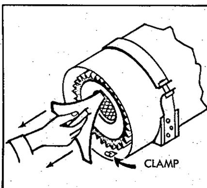
**C. Pull out locking mechanism.**
