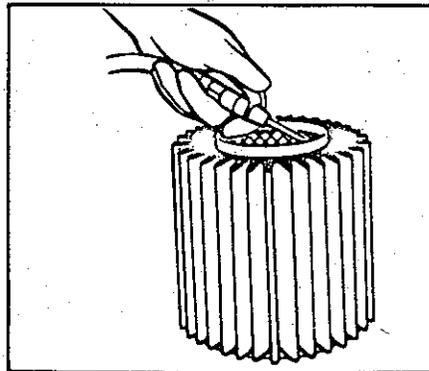
G. Blow off the inside of the cartridge again to remove any dirt on the clean air side that may have blown through when outside was cleaned.
