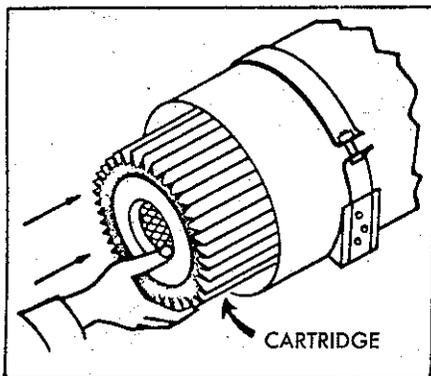
H. Replace cartridge in can. **Caution:** Clean inside of can before replacing cartridge.
