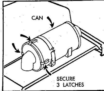
K. Replace cover on can by securing the (3) latches.
