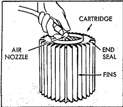
E. Blow off the inside of the cartridge with 100 lbs. compressed air.
