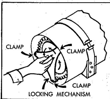
**B. Release locking mechanism by turning handle counter clockwise and turn until mechanism is disengaged from clamps.**
