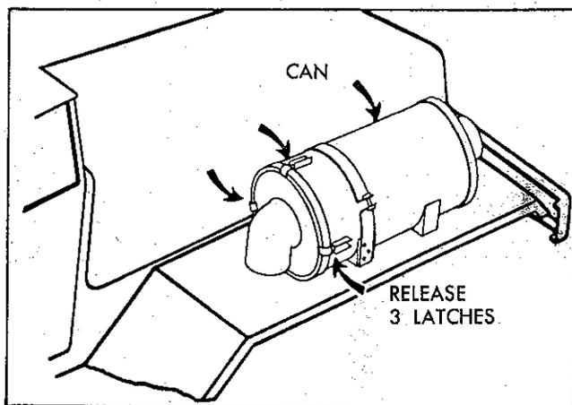
**A. Remove cover by unlatching the three assemblies that hold the cover to the can.**
