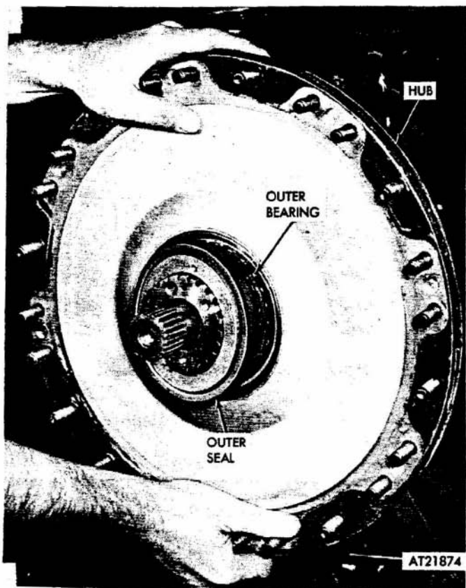
Figure 2-221. Loosening outer bearing and seal
