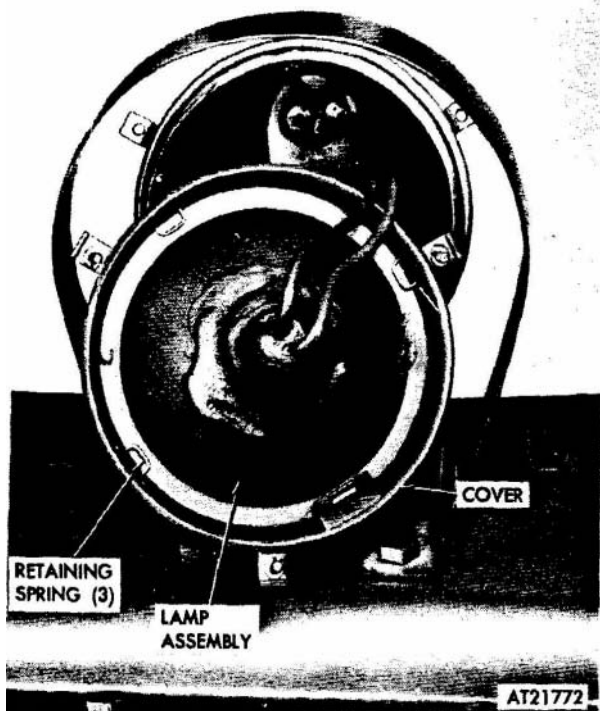
Figure 2-120. Blackout headlight lamp replacement.
