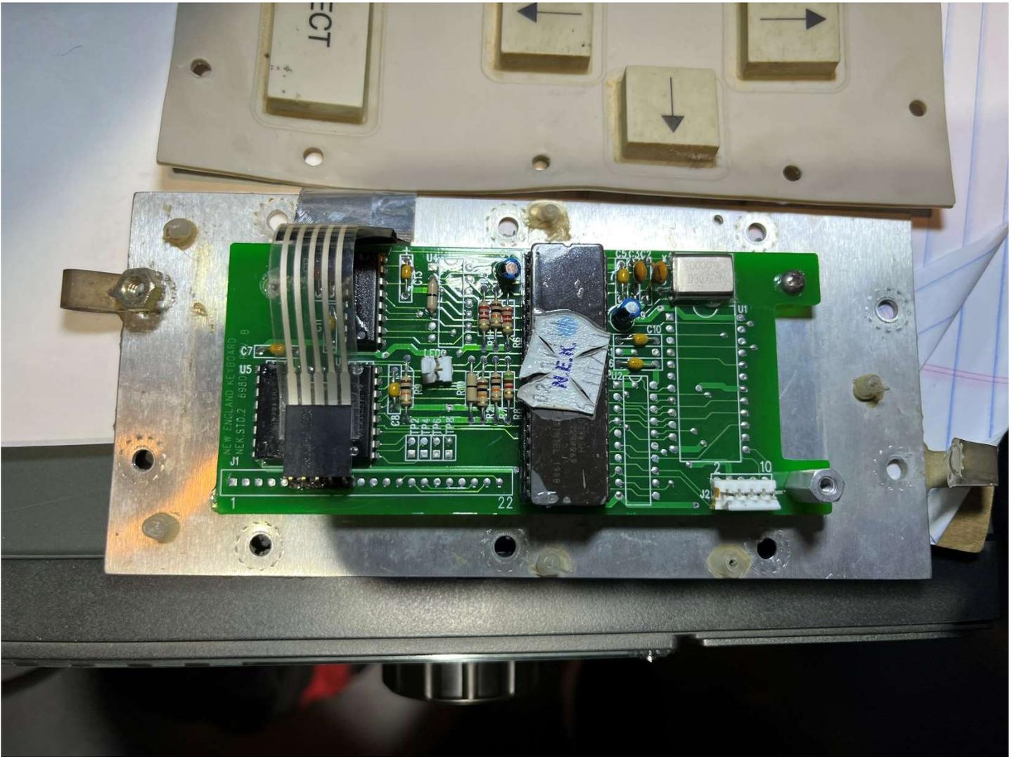
You can see the shiny conformal coating sprayed and/or dipped over the entire PCB.
