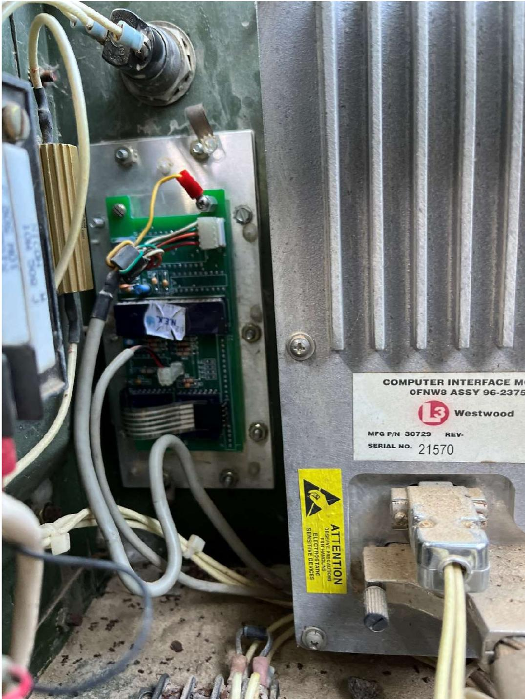
The keypad went back in surprisingly easy and most of the 10 screws around the perimeter were easy to fasten. Be sure to tie-wrap the cables to other nearby cables so that they do not vibrate too much. Also keep them away from the power resistors on the side wall so that they do not get charred or melted.
