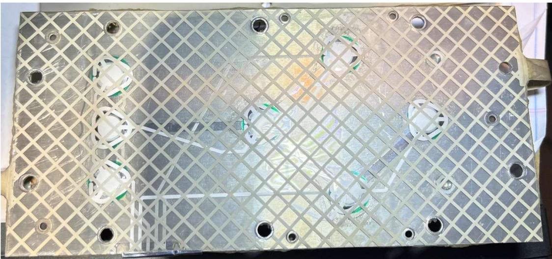
I disconnected the flex cable running from the keypad to the PCB and verified with an ohmmeter that the keys made a proper connection. You can do this by choosing any two pins and pressing buttons until you get a low-resistance connection
