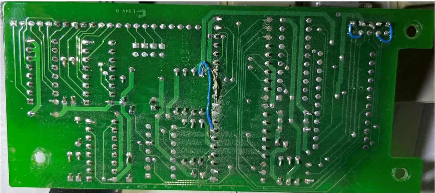
The workmanship for the blue wire in the middle of the PCB is poor. There may have been a short from this wire to a pad underneath. I had problems getting the keypad to work until I pried the blue wire up from its glue trail and moved it over slightly to the left as shown above.
