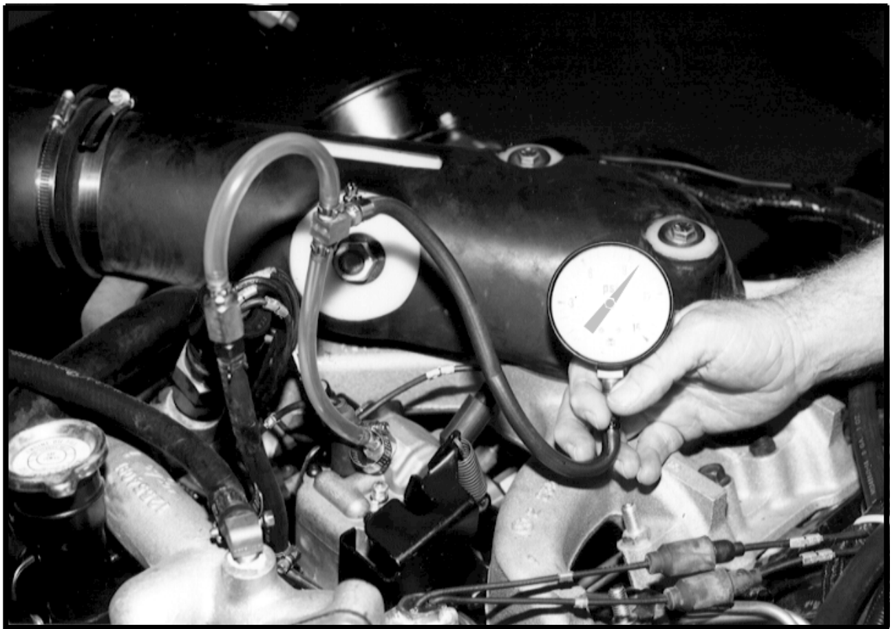
Fuel Return Pressure Check
