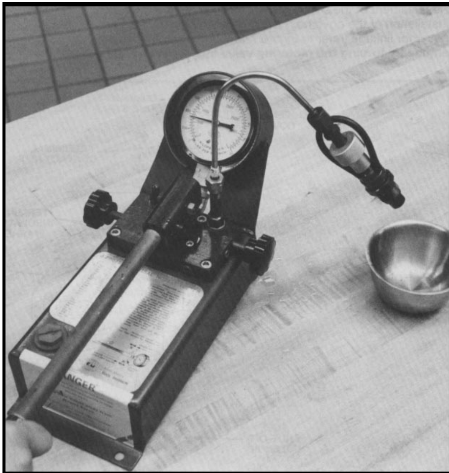
Injection Nozzle Testing
