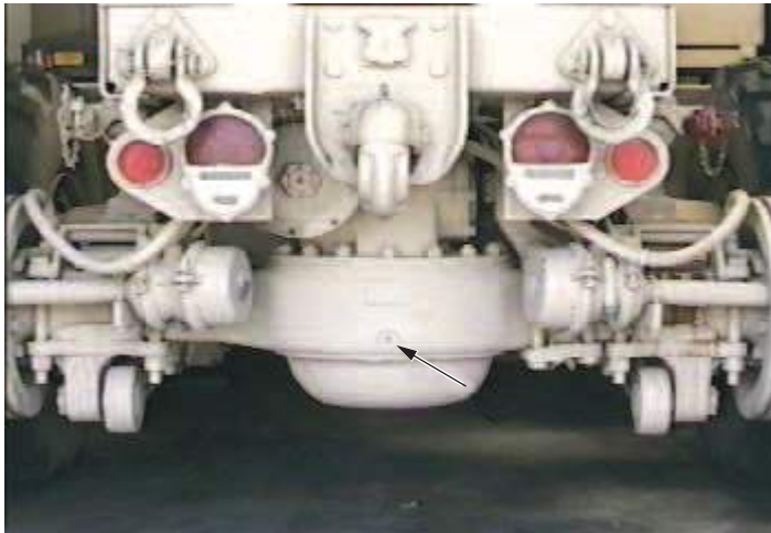
Figure 3. Differential Lubrication Level.
