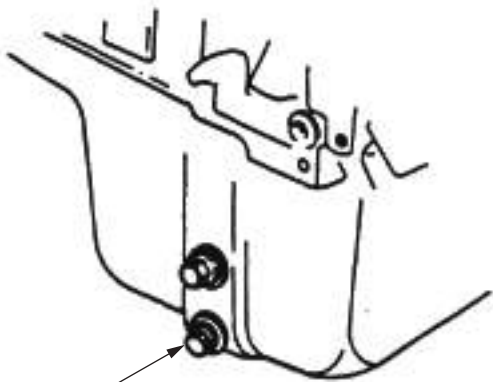
CRANKCASE DRAIN M939A2
