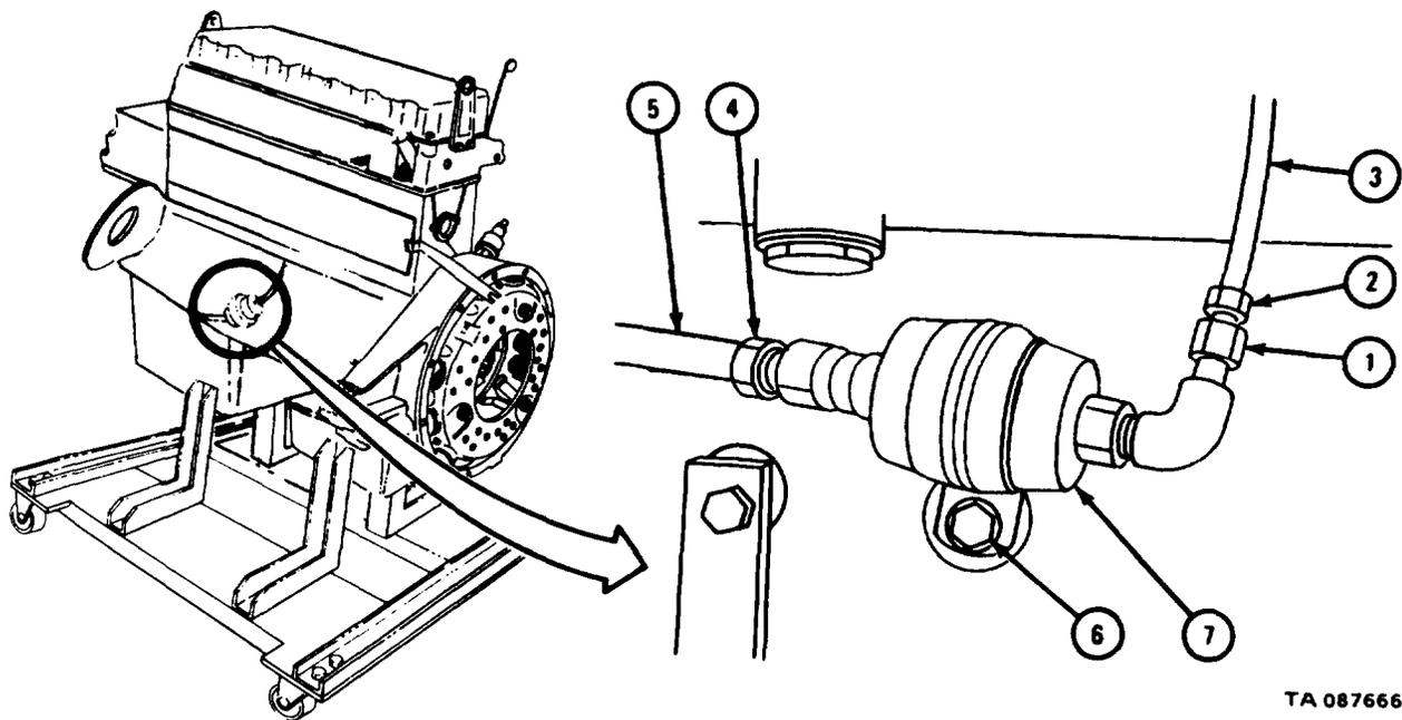
d. Top Mounted-Uncovered Flame Heater Ignition Unit and Fuel Pump.
