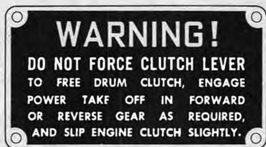
Figure 36. Front winch clutch lever warning plate—all models with front winch.
