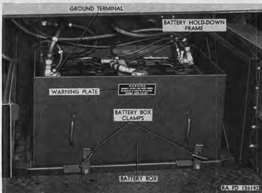
Figure 181. Battery installation.
