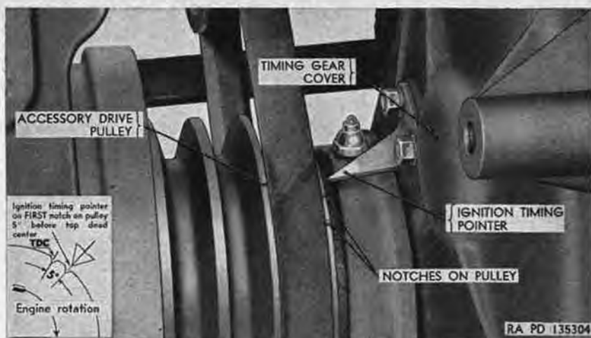
Figure 128. Ignition timing indicator.
