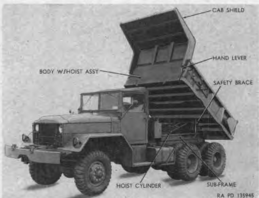
Figure 94. Dump truck M51 with body in raised position.
