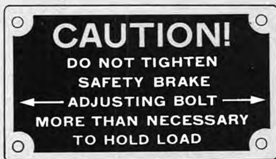
Figure 37. Front and rear winch automatic brake caution plate—all models with winch.
