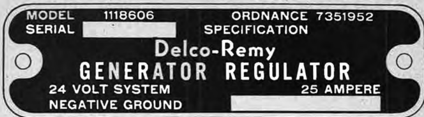
Figure 24. Generator regulator nameplate.
