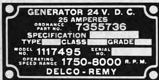
Figure 23. Generator nameplate.
