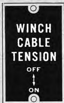
Figure 43. Rear winch cable tension lever instruction plate—model M62.
