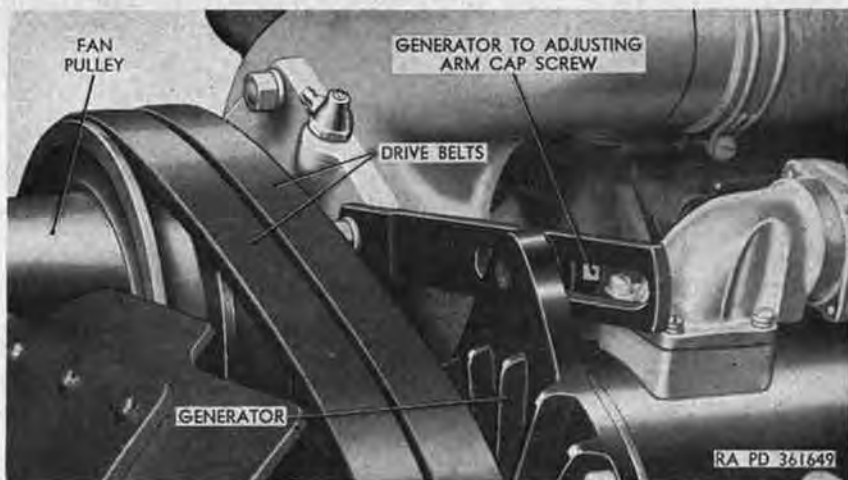
Figure 164. Drive belts installed on fan pulley.
