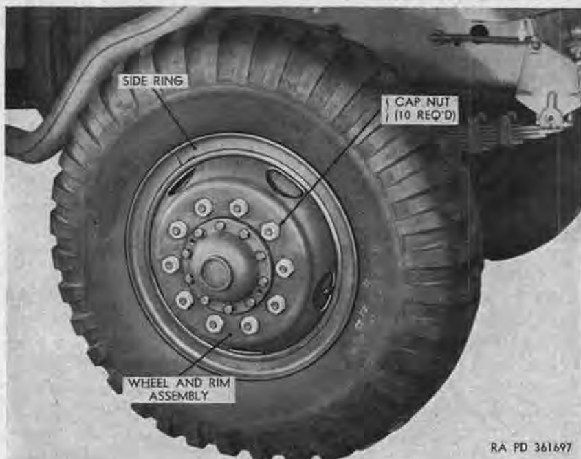
Figure 256. Wheel and tire assembly with snap-on-type side ring (11:00 X 20 tires)
