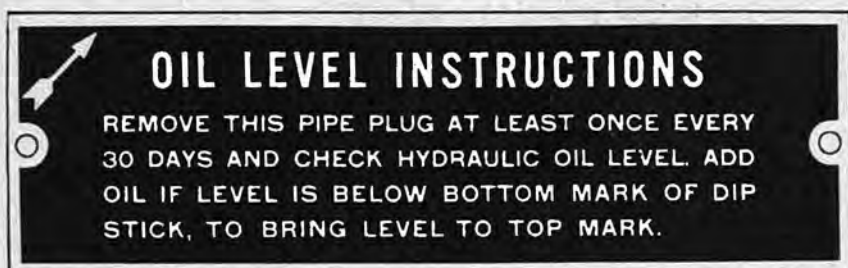
Figure 55. Reservoir oil level instruction plate—models M62 and M246.
