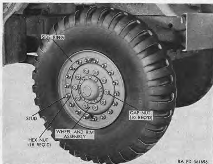
Figure 255. Wheel and tire assembly with bolted-on-type side ring (14:00 X 20 tires)
