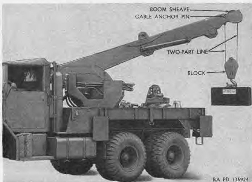
Figure 83. - Crane rigged with two-part line (M62).
