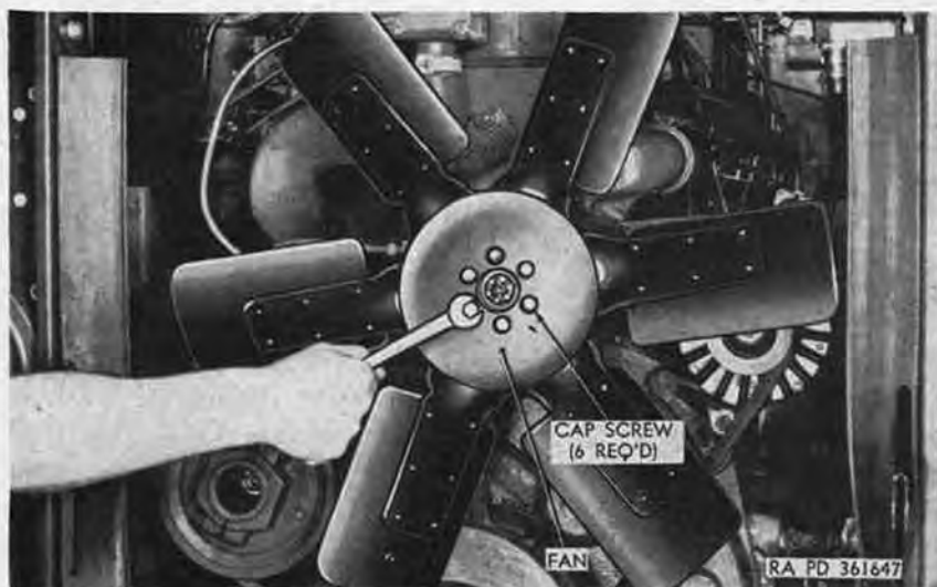
Figure 165. Front view of fan installed on fan pulley.
