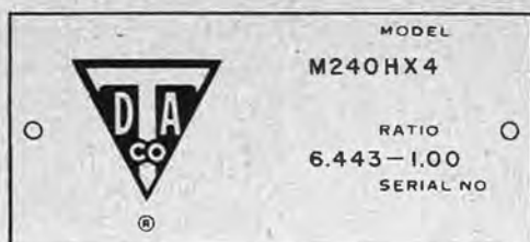
Figure 27. Rear axle nameplate.
