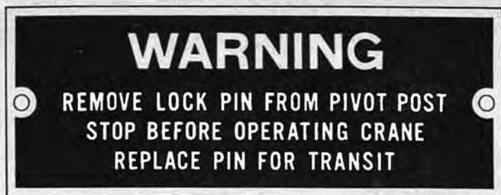
Figure 62. Hydraulic crane pivot post lockpin warning plate—model M246.
