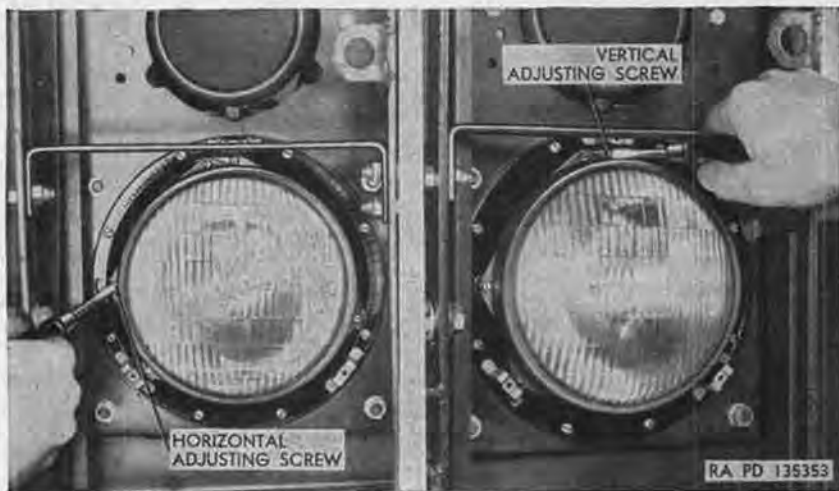
Figure 184. Adjusting headlight.
