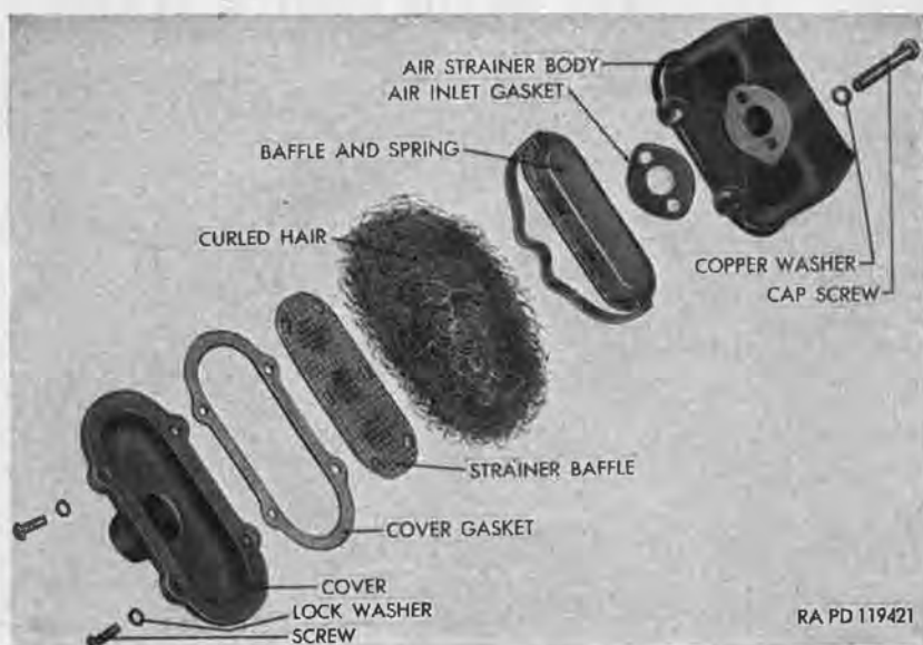
Figure 251. Air-compressor air strainer—exploded view.
