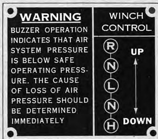
Figure 31. Low air pressure warning and winch control data plate.
