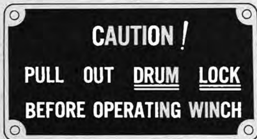
Figure 35. Front winch drum lock caution plate—all models with front winch.
