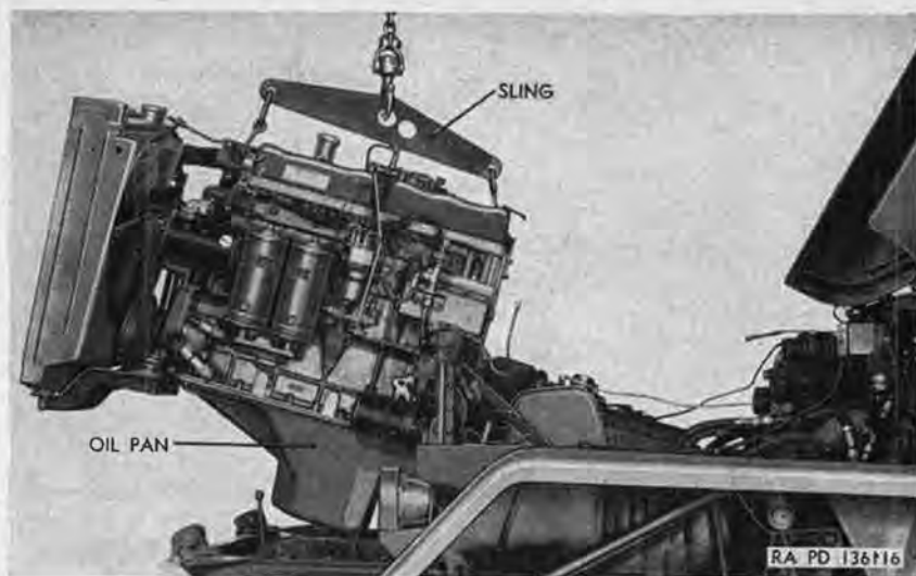
Figure 150. Lifting power plant from truck.
