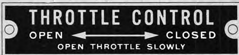
Figure 41. Winch throttle control lever instruction plate—model M62.
