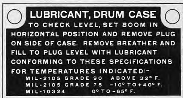
Figure 54. Cable drum gearcase lubricant plate—models M62 and M246.
