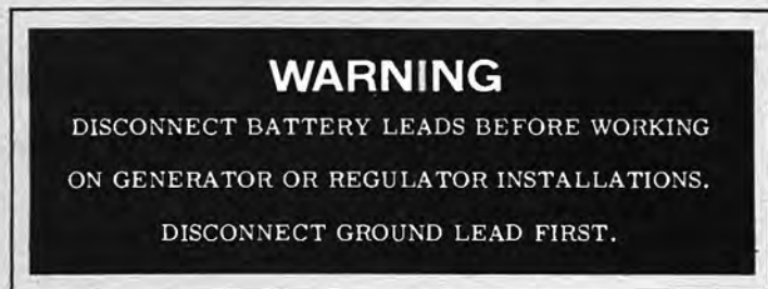
Figure 29. Battery disconnect warning plate.
