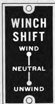
Figure 40. Rear winch shifting instruction plate—model M62.
