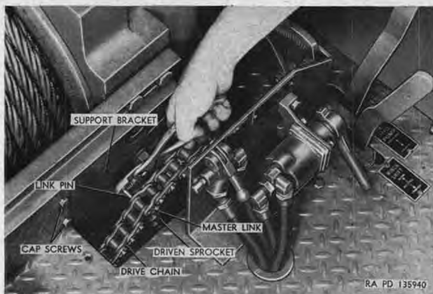
Figure 281. Separating rear winch drive chain M62.
