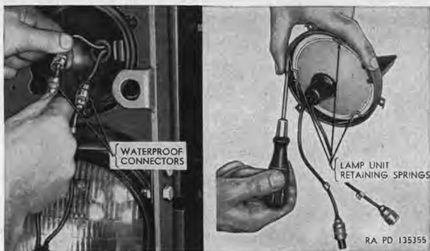
Figure 187. Removing sealed-beam.
