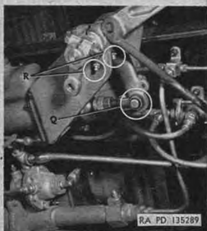
Figure 108. Localized lubrication points (H-R).
