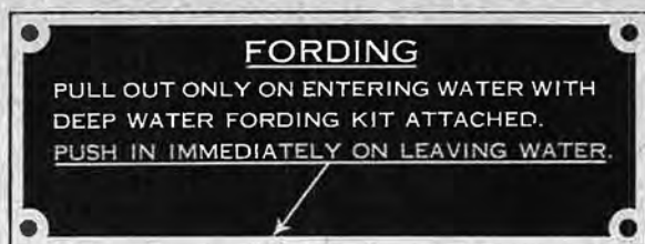
Figure 30. Crankcase ventilating shut-off valves data plate.
