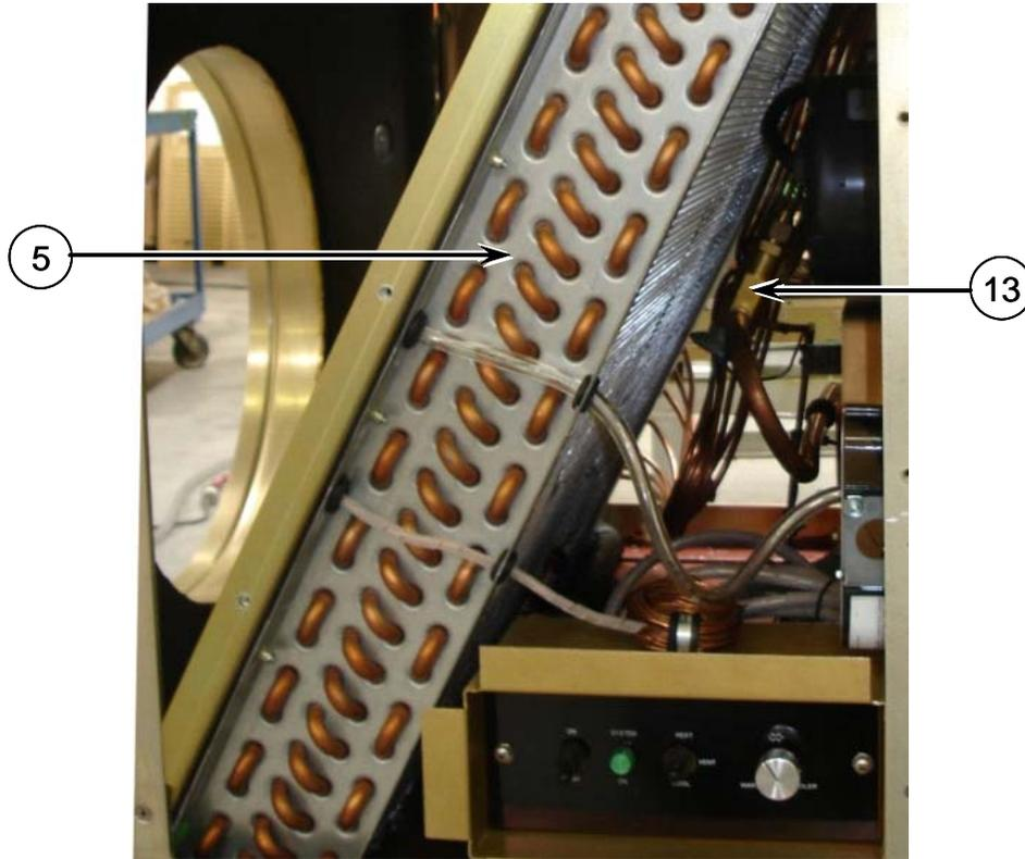
**Figure 8-6 Evaporator Side Components, Forward**
