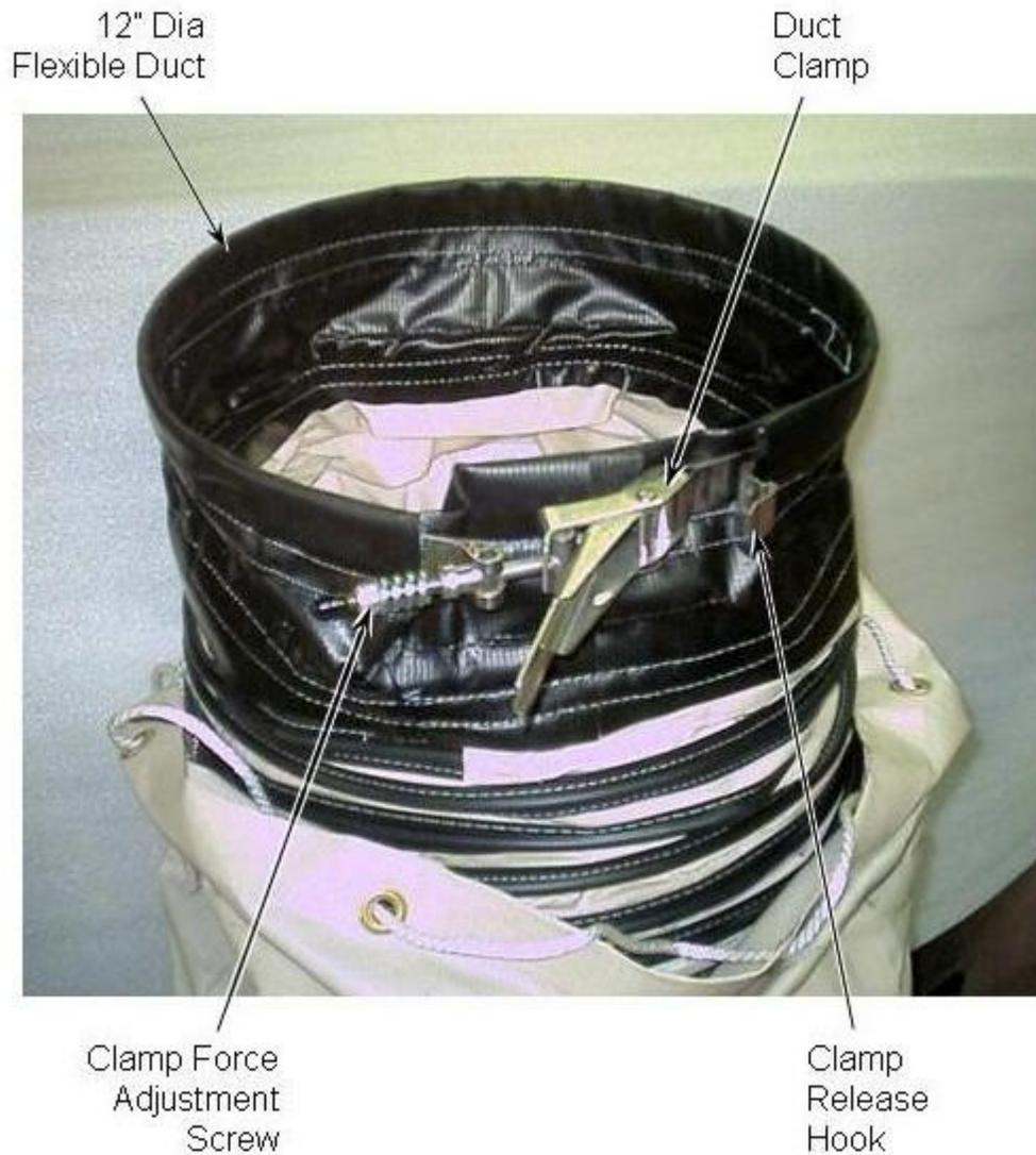
**Figure 4-2 Duct Attachment, Closed**
