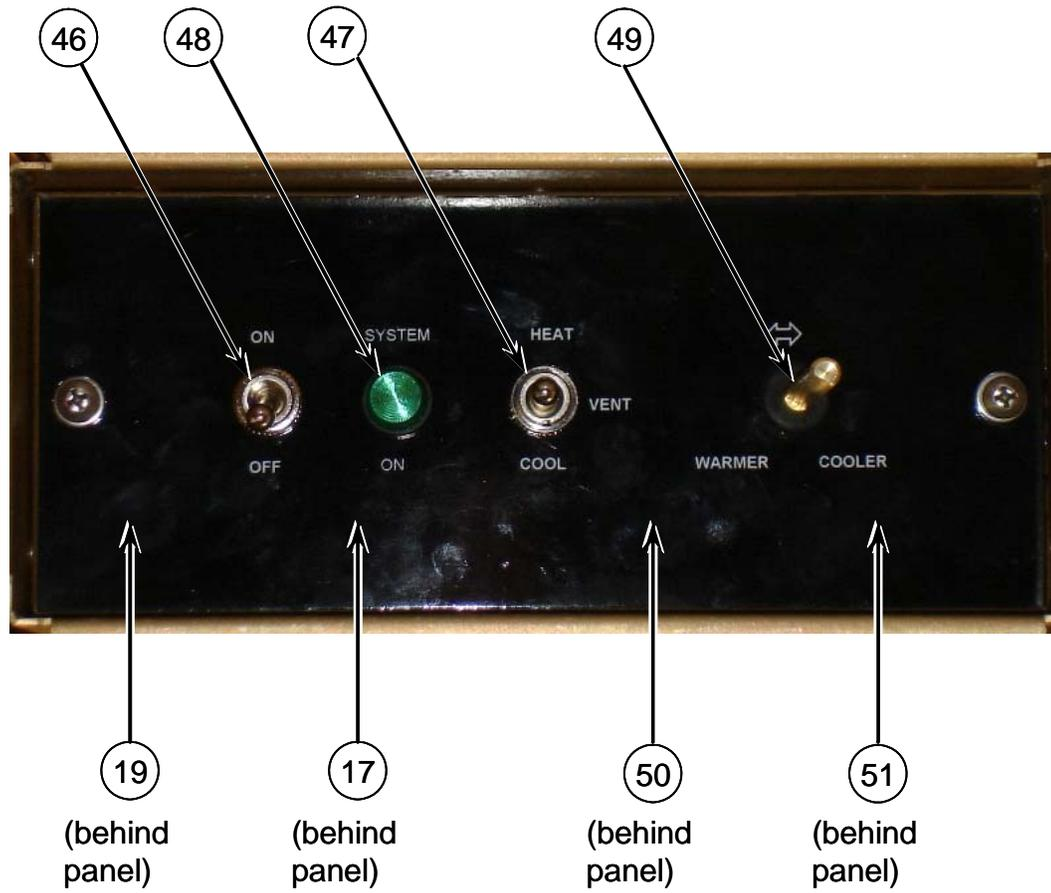
**Figure 8-10 ECU Control Panel Box (Panel Removed)**
