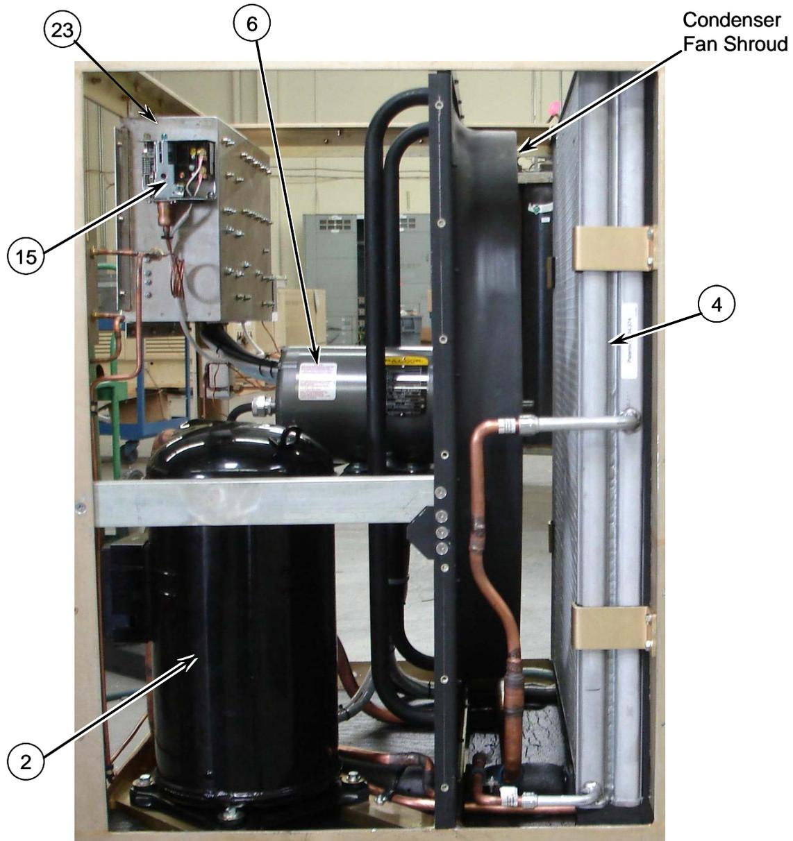
Figure 8-3 Condenser Side Components, Aft
