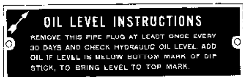
Figure 57. Reservoir oil level instruction plate—models M62 and M246.
