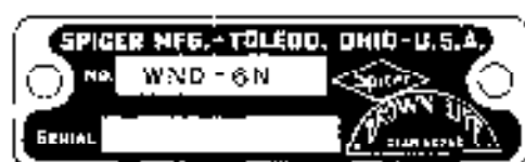
Figure 32. Power-take off nameplate—Not only.
