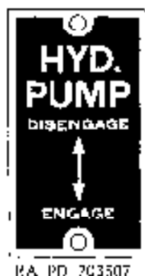
Figure 48. Hydraulic pump control lever instruction plate—model M62.
