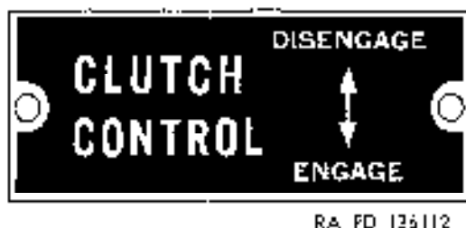
Figure 47. Clutch control lever instruction plate—model M62.
