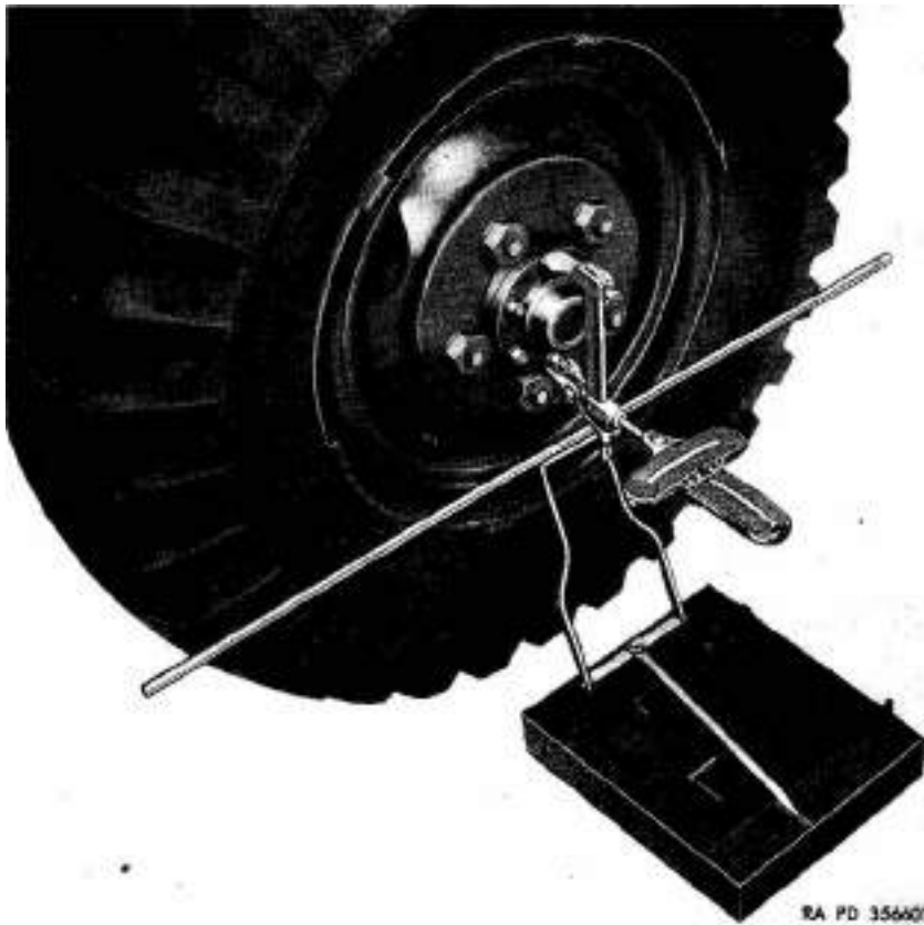
Figure 71. Checking front axle camber, caster, and pivot pin inclination with wheel alinement indicator.
