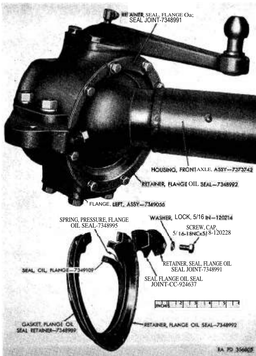
Figure 57. Flange oil seal retainer and related parts.
