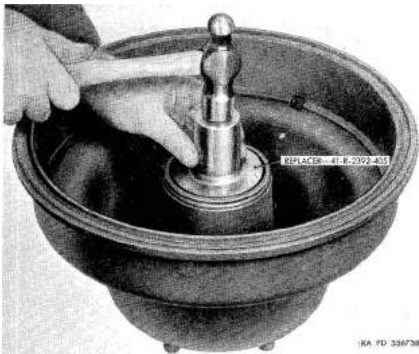
Figure 56. Installing hub bearing oil seal assembly.
