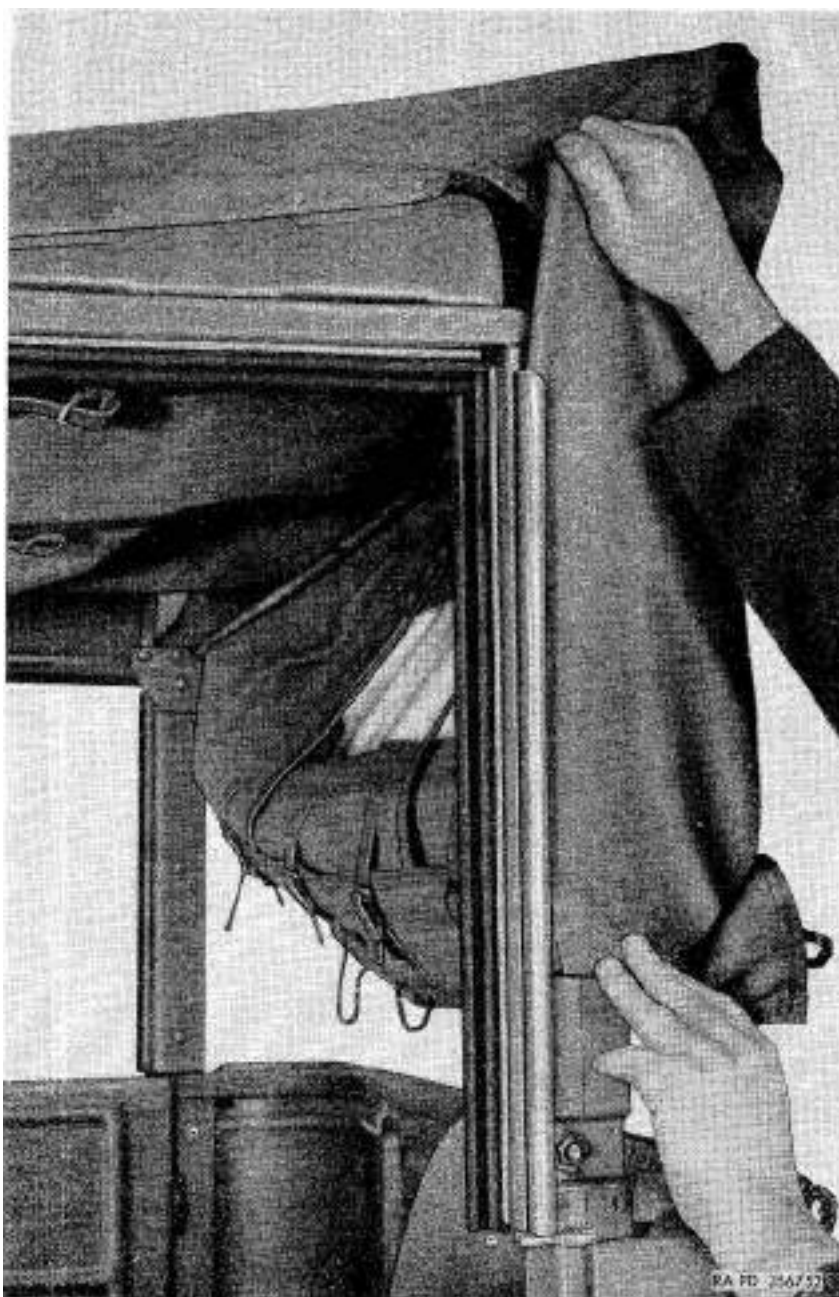
Figure 19. Removing top cover from top side rail supports.
