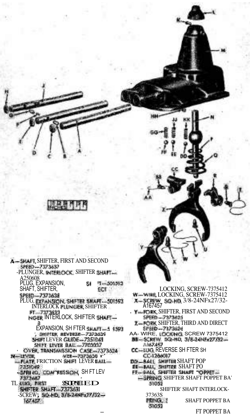
Figure 111. Transmission case cover assembly—exploded view.
