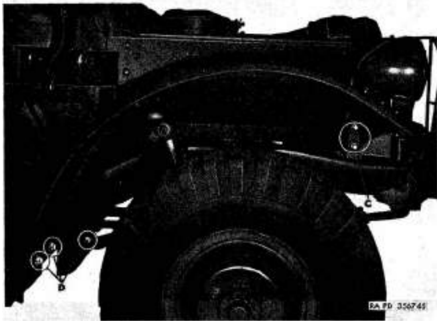
Figure 12. Fender and radiator guard assembly disconnect points.
