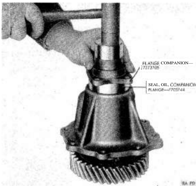
Figure 131. Installing companion flange oil seal.
