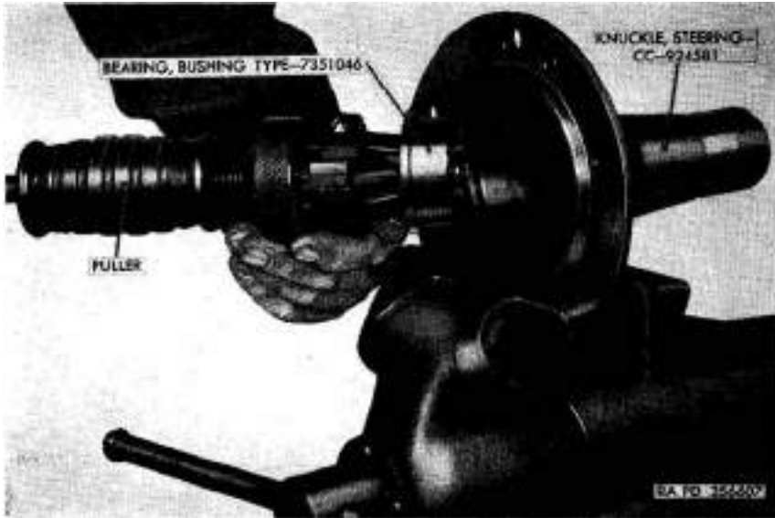
Figure 60. Removing bushing-type bearing from steering knuckle with a puller.
