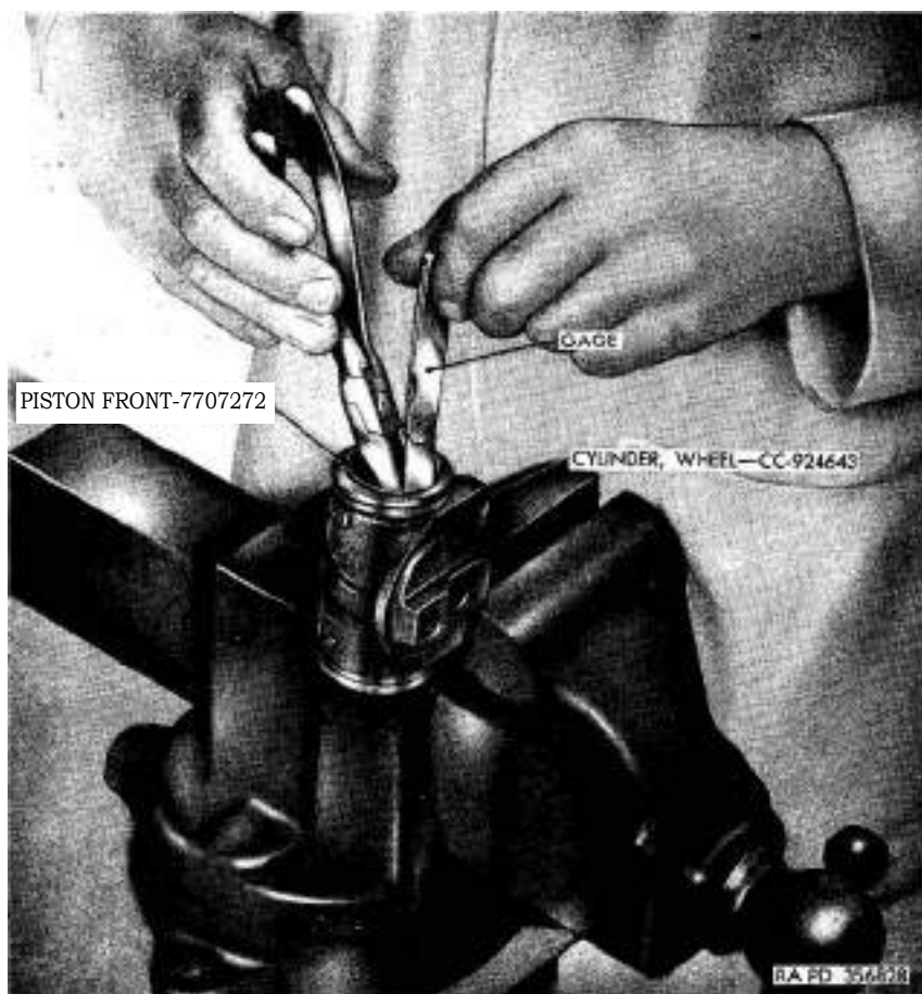
Figure 153. Checking clearance between wheel cylinder and piston with thickness gage.
