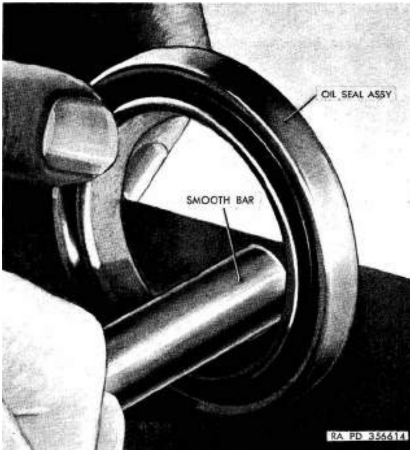
Figure 55. Rolling leather oil seal with round smooth bar.
