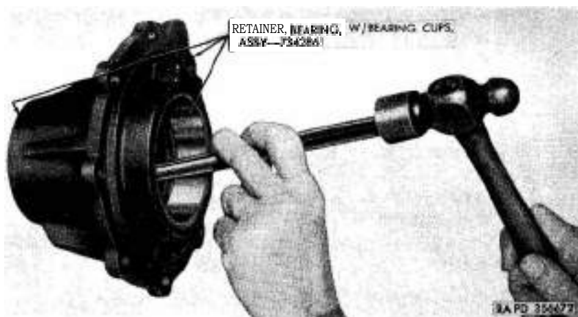
Figure 126. Removing bearing cups from bearing retainer.
