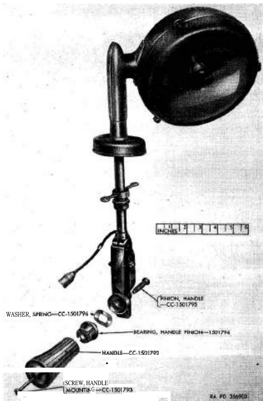
Figure 231. Spot light handle and related parts.
