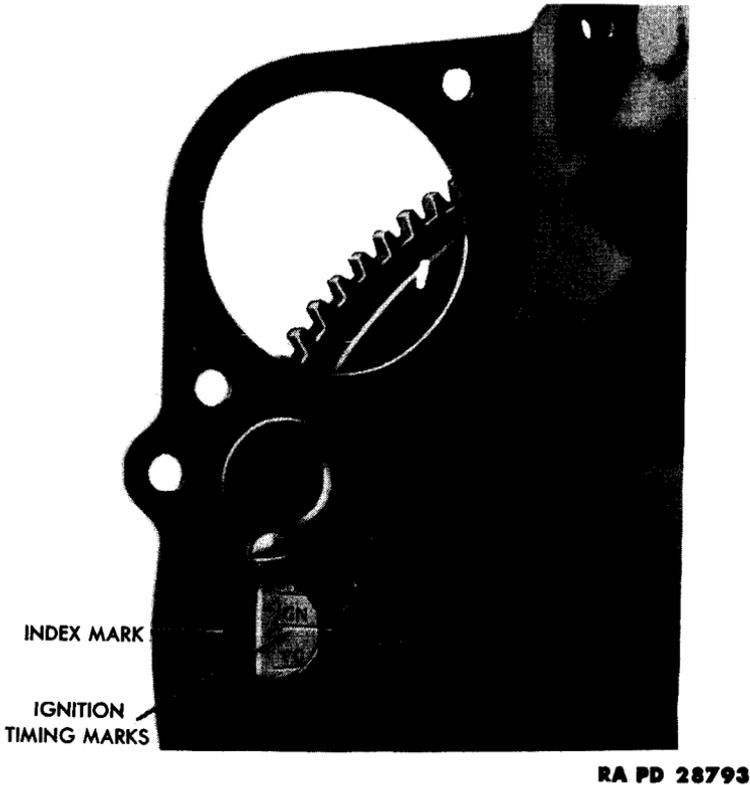
**Figure 42 — IGN Timing Marks on Flywheel**
