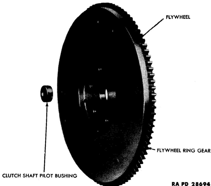
*Figure 31 — Flywheel Ring Gear and Pilot Bushing*
