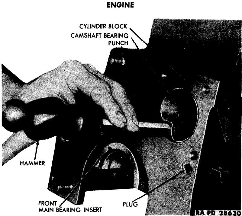
**Figure 14 – Driving Camshaft Bearing from Cylinder Block**
