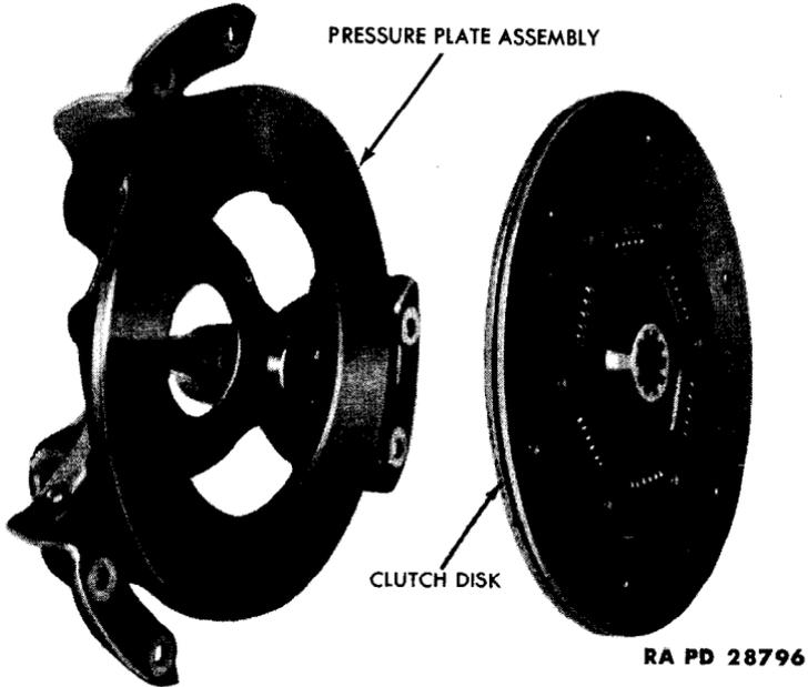
Figure 46 — Clutch Disk and Pressure Plate
