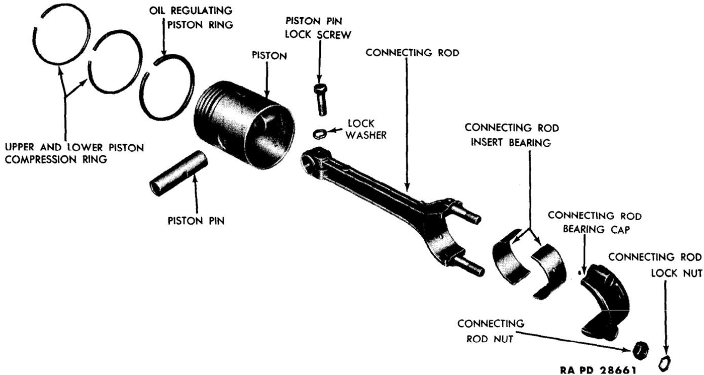
Figure 22 – Connecting Rod and Piston Assembly, Disassembled
